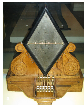
The Cooke and Wheatstone electric telegraph can transmit letters with the use of 5 needles which point to the transmitted letters. CC BY-SA 4.0 by Geni on Wikimedia Commons
